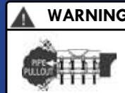
**WARNING** This is a non-restraining product. If pipe pullout can occur, proper anchoring of the pipe joint is required. Failure to anchor the pipe could result in the escape of line content, and may cause property damage, serious injury or death.
